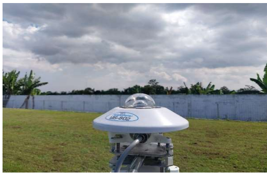
Figure 3. Measurement of GHI using a Pyranometer
